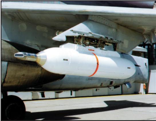
AIM-9X CTU on Wing Pylon
